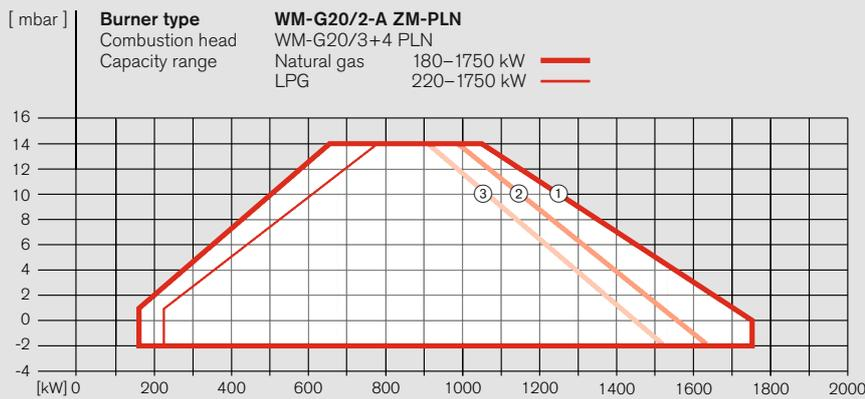
Capacity graphs for gas burners certified in accordance with EN 676.
