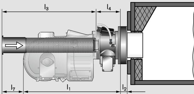
Installation aid – minimum clearance with spacer ring
