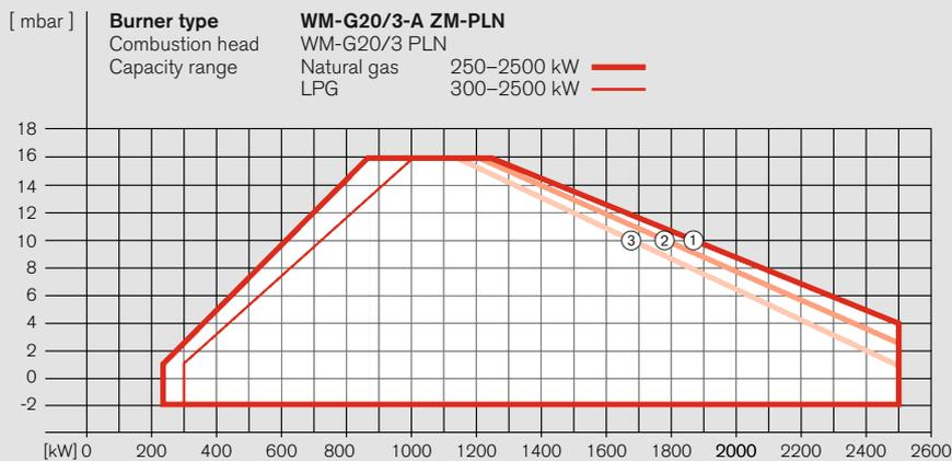
**Determining load point dependent on excess air**
