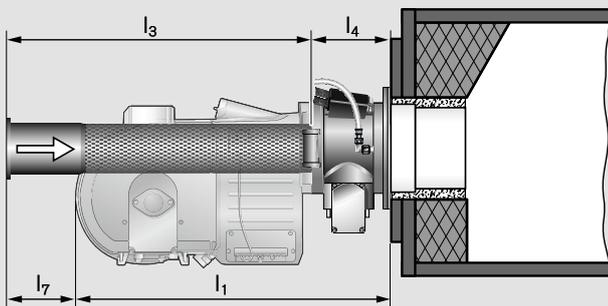
Installation aid – minimum clearance without spacer ring
