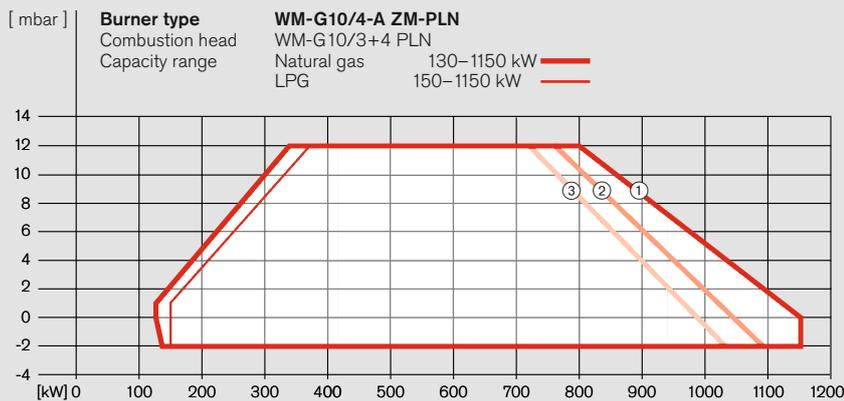
**Determining load point dependent on excess air**
