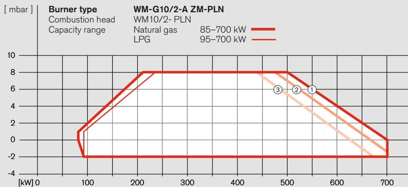
**Determining load point dependent on excess air**
