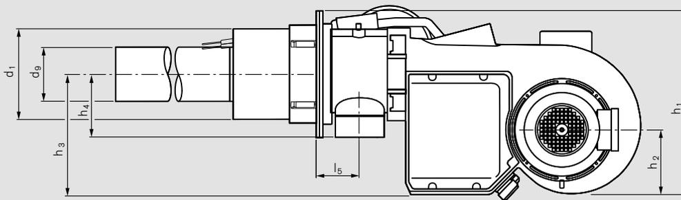
Mounting-plate drilling dimensions
