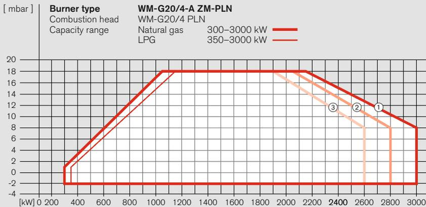
Capacity graphs for gas burners certified in accordance with EN 676.
